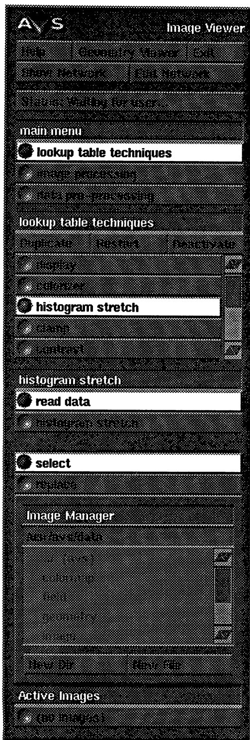
Figure A-3. Control Panel for 'histogram stretch' Technique (pull-down menu, accessed via the small square in the window's title bar — see next section.)
